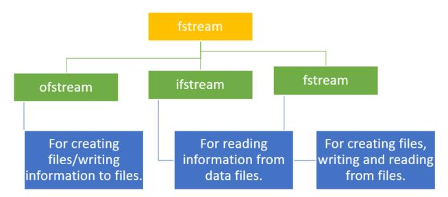
**Ofstream**: This data type represents the output file stream and is used to create files and to write information to files.
